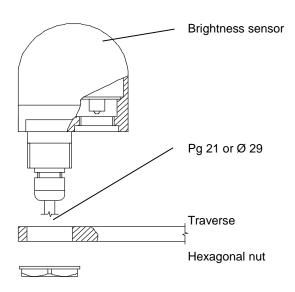
The unit can be fitted e.g. to a mast tube, beam with a Pg 21 threaded hole or onto the bracket available from Thies Clima\*. The cable (type: LiYCY) is threaded through the hole and the brightness transmitter is connected to it by means of a hexagonal nut (SW 36). The installation is vertical.
