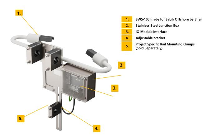
Note: The VIS-KIT-NAI-SWS100 must be fastened to the railing with three Stauff tube clamps of the heavy series (DIN 3015 part 2), size 4 – 6 (project specific).
