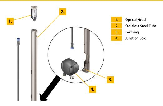
Note: All housing components including the cable glands satisfy the IP67 degree of protection requirements according to IEC 60529. During connection and assembly, ensure that no moisture or dirt penetrates into the open socket.
